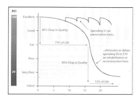
If intervention is delayed the deterioration curve becomes increasingly steep and the cost and scale of maintenance required in increased in a non-linear manner. Under investment causing the delay of interventions leads to rapid and non-linear deterioration. Routine maintenance is replaced with carriageway reinstatement or even in extreme cases reconstruction of most or all of the layers which make up the carriageway. Extended delays in
